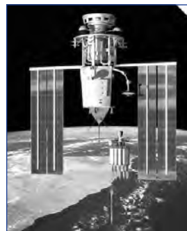
Figure 12-2 KEIs might involve de-orbiting tungsten rods at hypersonic velocities.
