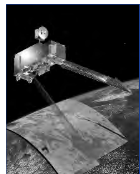
Figure 6-4 Illustration of Terra's MOPITT device scanning the earth for methane.
